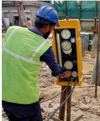
Fig. 5. Pressuremeter test in progress.
