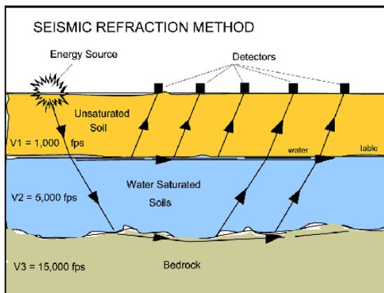
Fig. 2. Schematic sketch of Seismic refraction test
