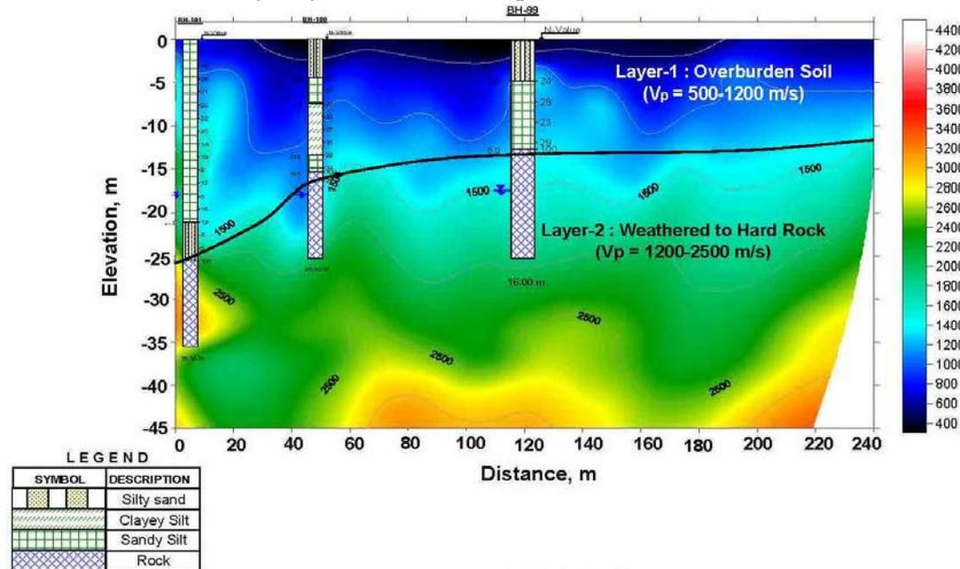
Fig. 4. Seismic profile and borehole data at Station 1 (RK Ashram)
