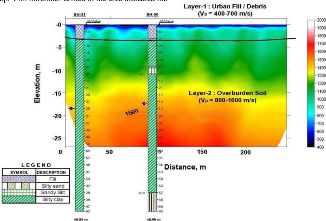
Fig. 6. Seismic profile and borehole data at Station 3 (Derawal Nagar)
