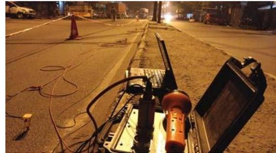
Fig. 3. Seismic refraction test in progress
