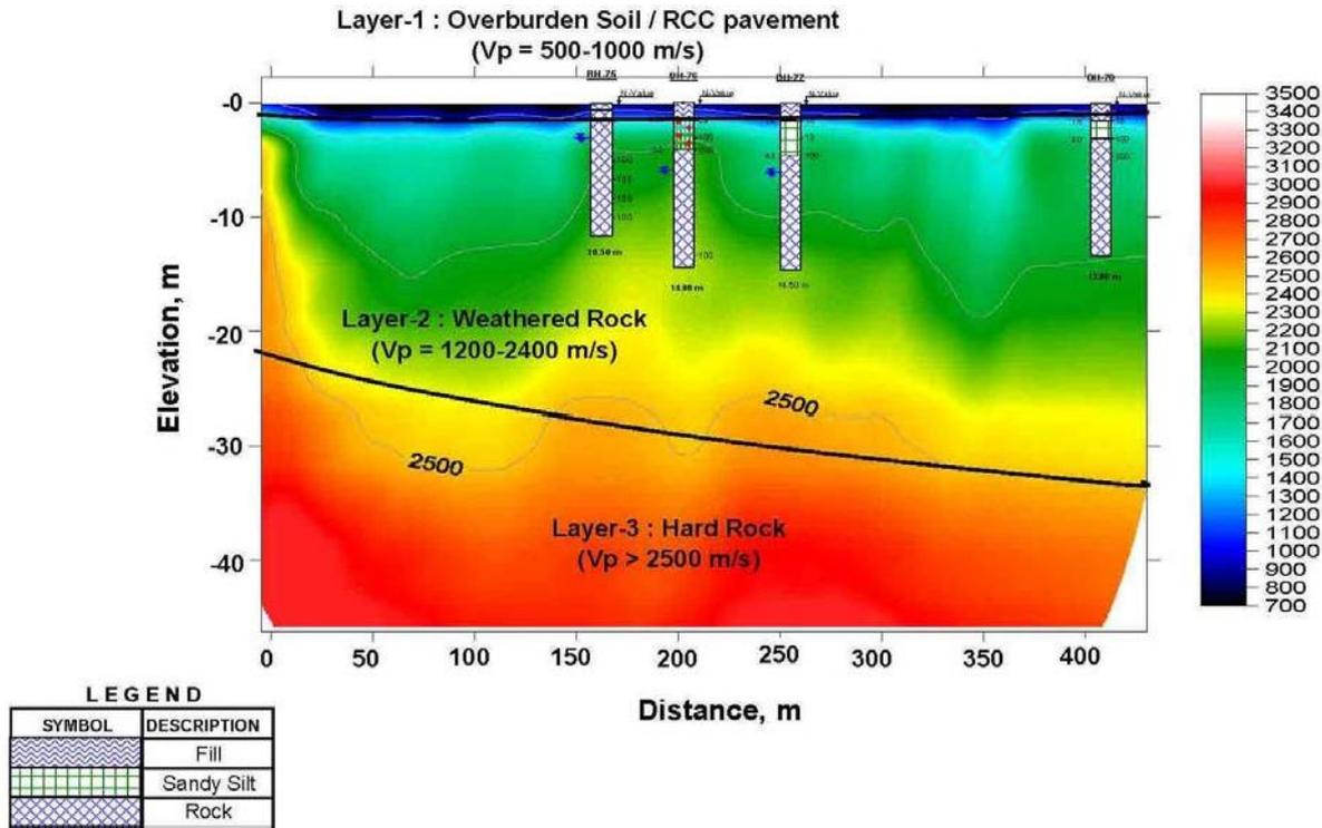
Fig. 5. Seismic profile and borehole data at Station 2 (Sadar Bazar)
