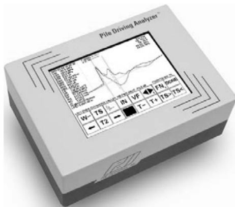
Fig. 6. Pile Driving Analyzer (PDA)
