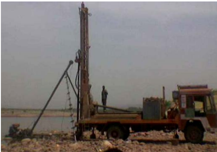
Fig.4: Odex & Percussion Boring
