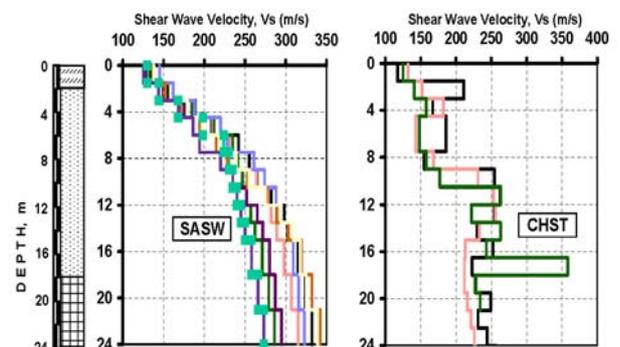
Fig. 3 : Shear Wave Velocity Tests
