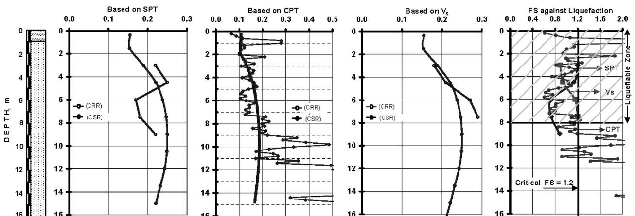
Fig. 5: Results of Liquefaction Analysis
