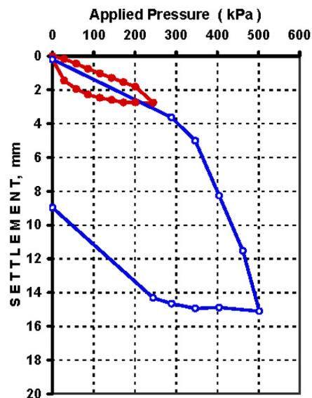
Fig. 9: Results of Load Test on Stone Column
