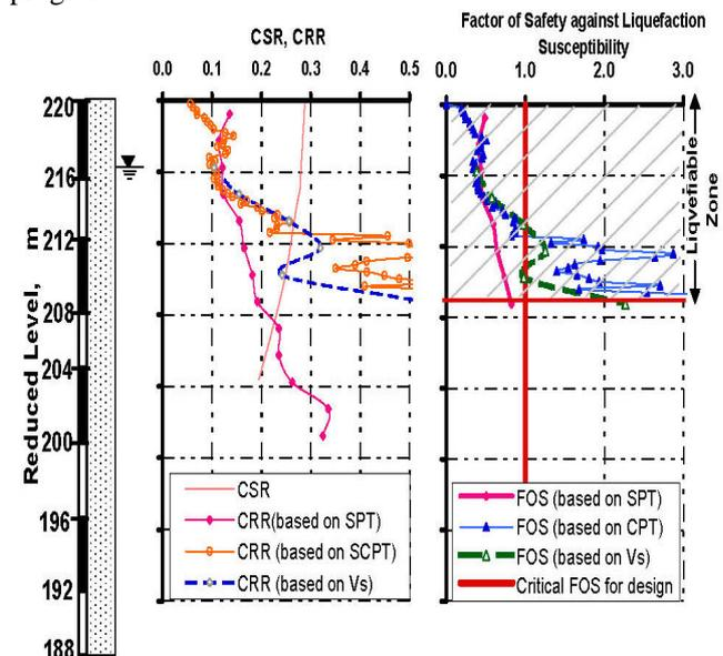
Fig. 4 CSR, CRR and Factor of Safety against Liquefaction
