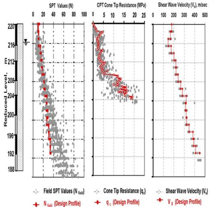
Fig. 3 SPT, qc and S Wave velocities profile
