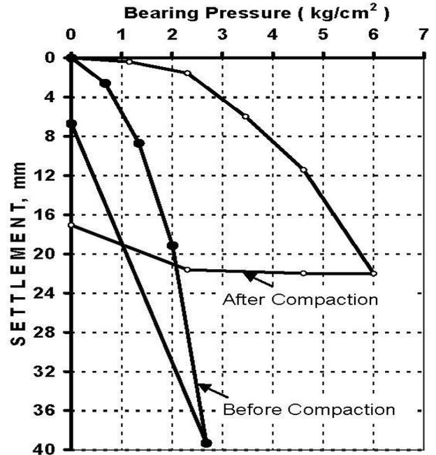
Fig. 7 Plate Load Tests before and after compaction
