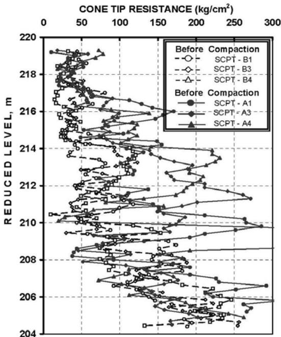
Fig. 6 Cone tip resistance before and after compaction (Boiler-I)
