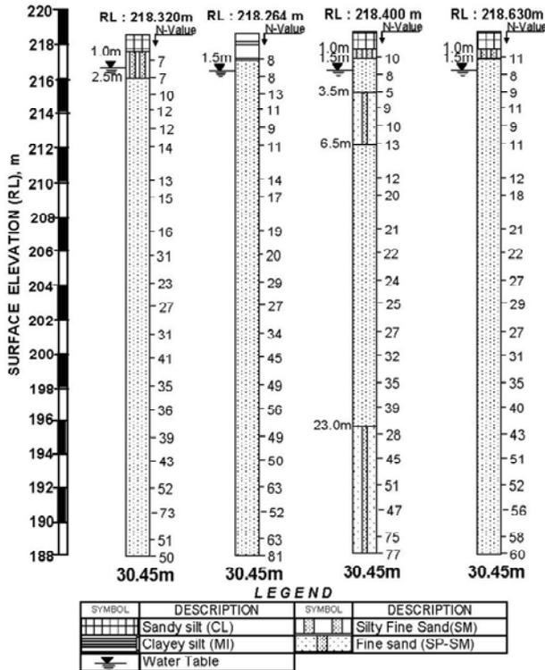
Fig. 2 Typical Borehole Data
